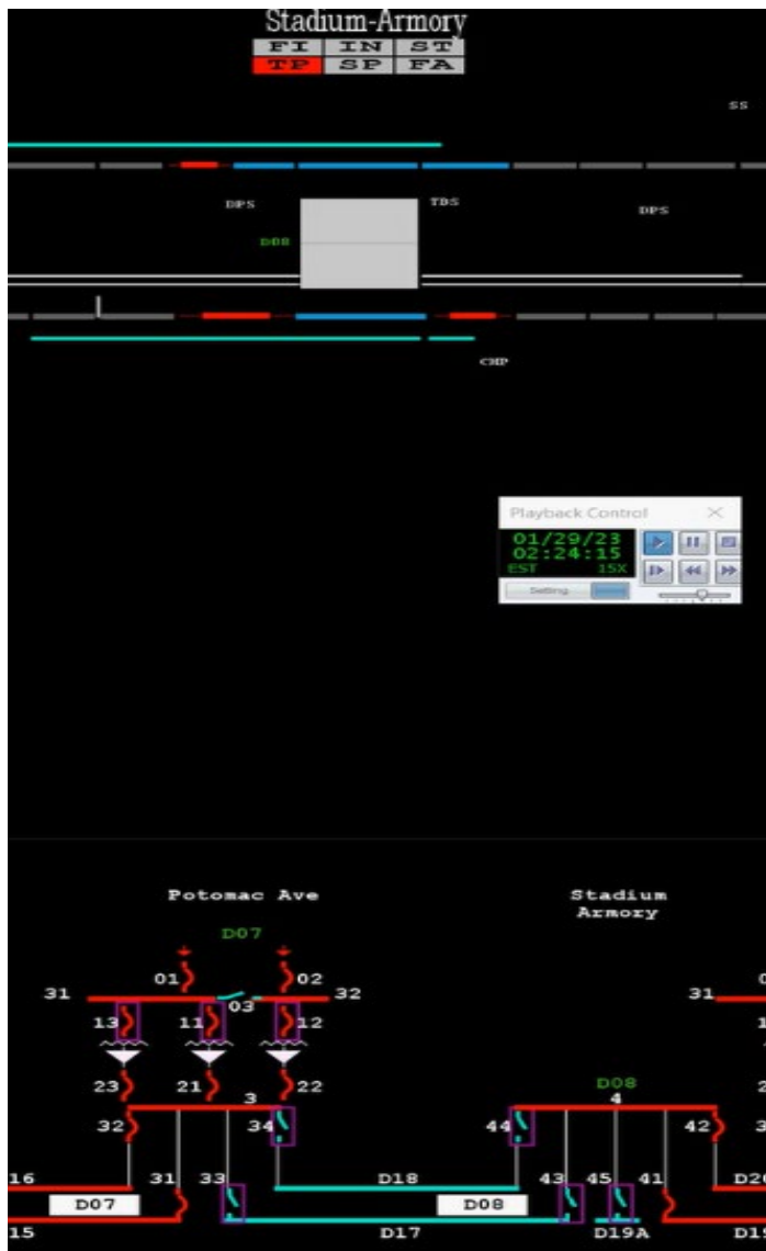
Figure 2 – AIMS one shunt Track 1, two shunts Track 2
