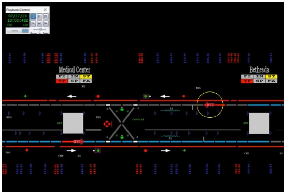
Figure 3 – AIMS depicting Train ID 105 stopped retrieved the RWIC and Track Inspector at approximately 10:03 hours.
