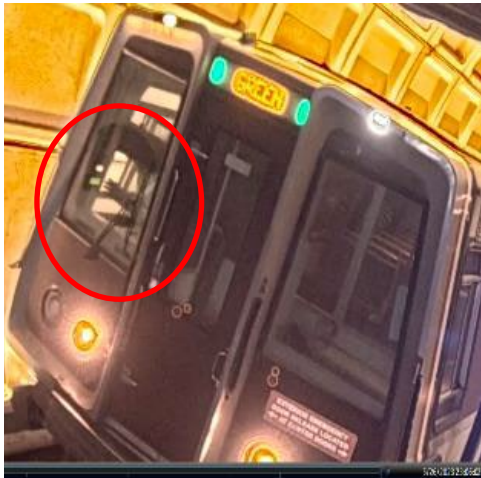
Figure 2 – Depicts the Train Operator pressing the door open button on Train ID 514 opening the train doors off-platform.
