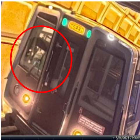
Figure 3 – Depicts the Train Operator's head out of the operator cab window on the off-platform side closing the train door.
