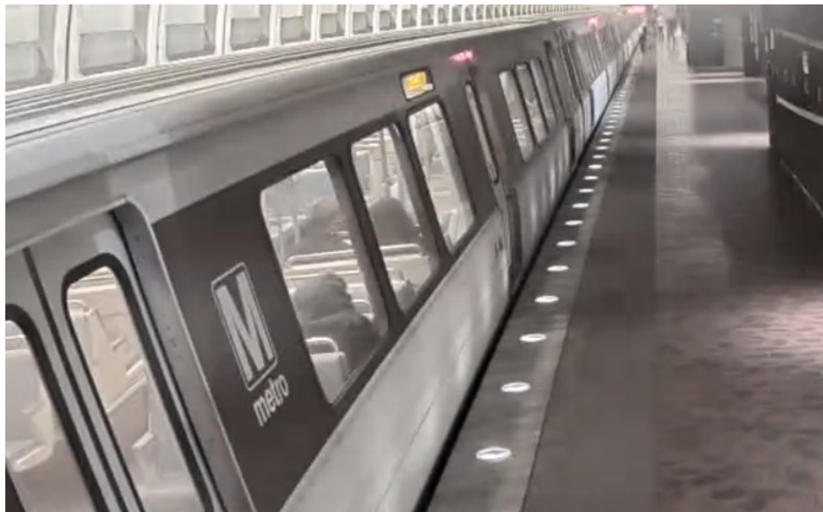
Figure 1 - Train ID 514 door signal lights illuminated, indicating train doors are open along consist. (Door closed on platform side)
