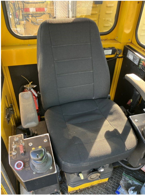
Image 9 - TC-07's main cabin and seat are not equipped with seat belts.
