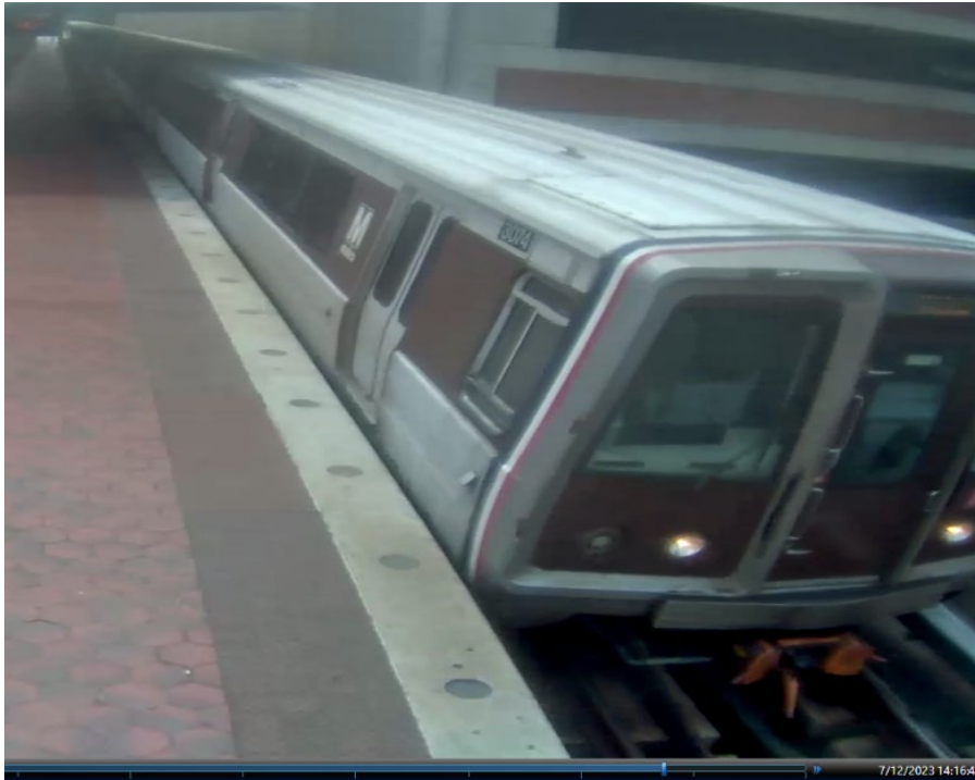
Figure 2 - depicts Train ID 402 lead car 3074 stopping approximately 30 feet from the 8-car marker at 14:16:42 hours.
