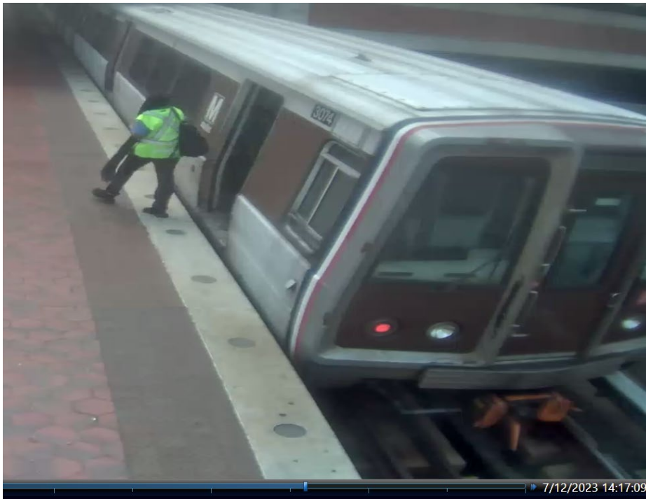
Figure 4 - depicts the Train Operator departing Train ID 402's lead car 3074 with the train doors open and the train not berthed at the 8-car maker.
