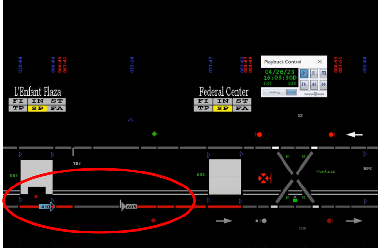
Figure 5 - AIMS Playback shows Train ID 605 moving against the normal flow of traffic. The displayed location is not exact and cannot be used to calculate distance.
