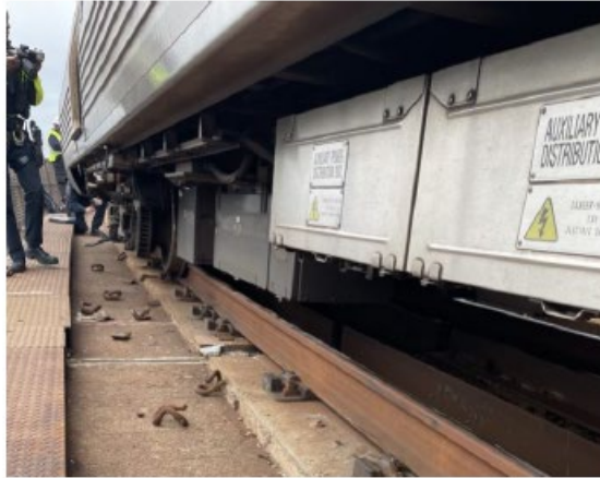
Figure 5: Derailed Left Wheel and Damaged fasteners & e-clips
