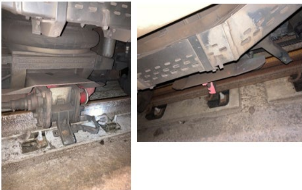
Image 2 - Missing Collector Shoe assembly from Train ID 308.
