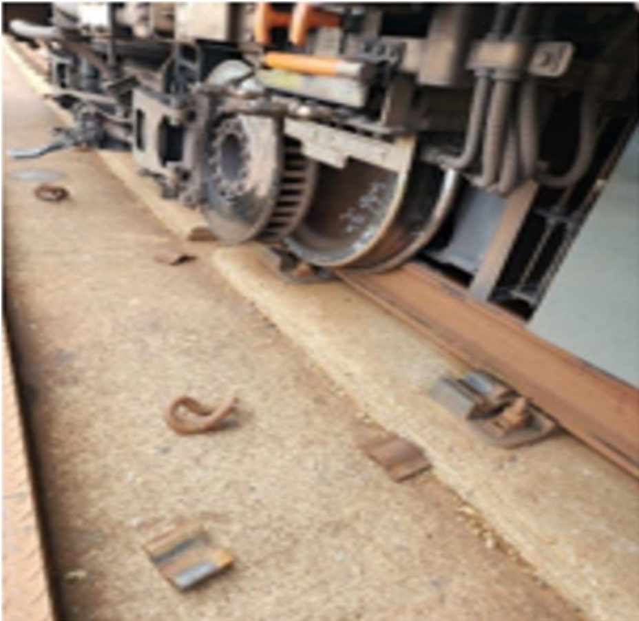
Image 3 - Derailment of Train ID 406 lead car
