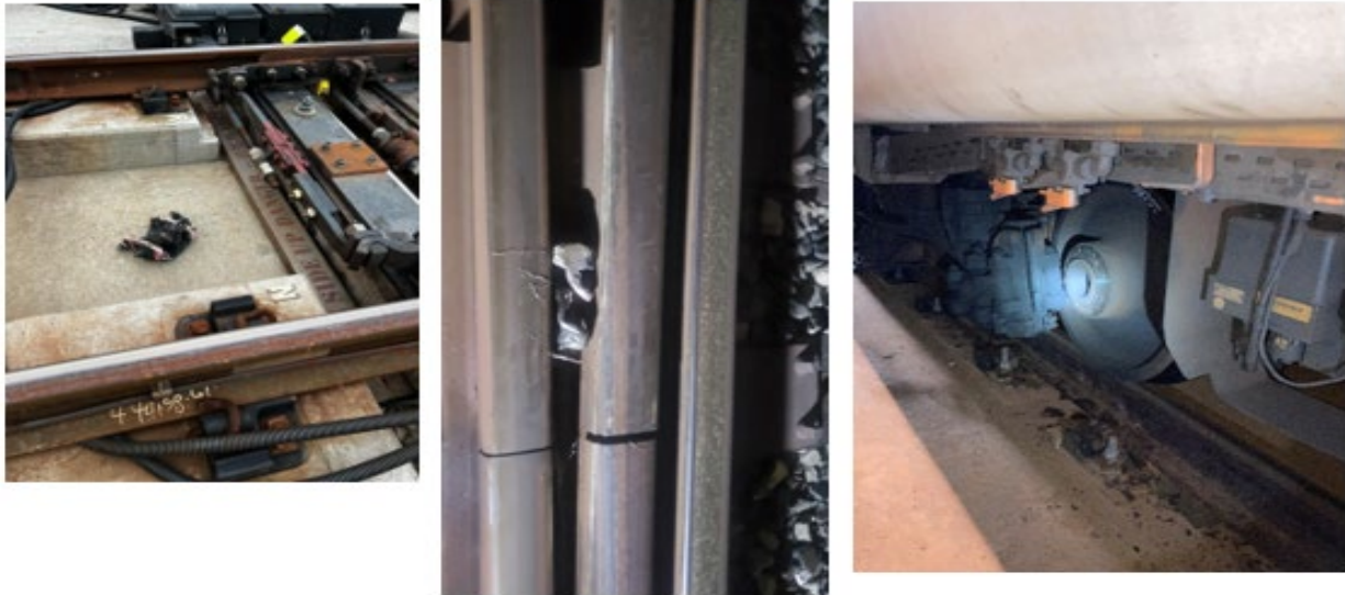
Image 1 – Collector Shoe parts and a missing brake disc from Train ID 308.
