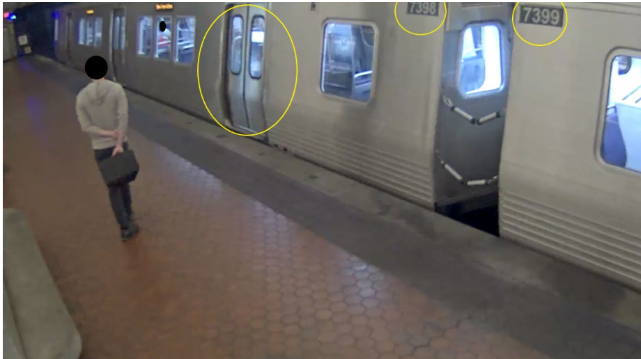
Image 6 - Train ID 909 stops at Federal Center Station at 09:18 hours for approximately 90 seconds and fails to service the platform, track 1.
