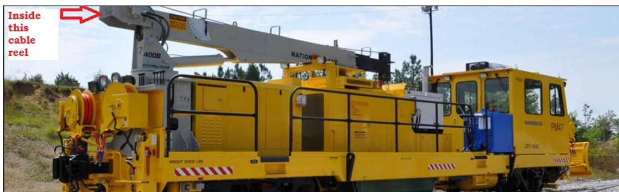
Figure 7 – depicts a vehicle similar to PM-578 and the boom from which the hydraulic fluid leaked (see arrow).
