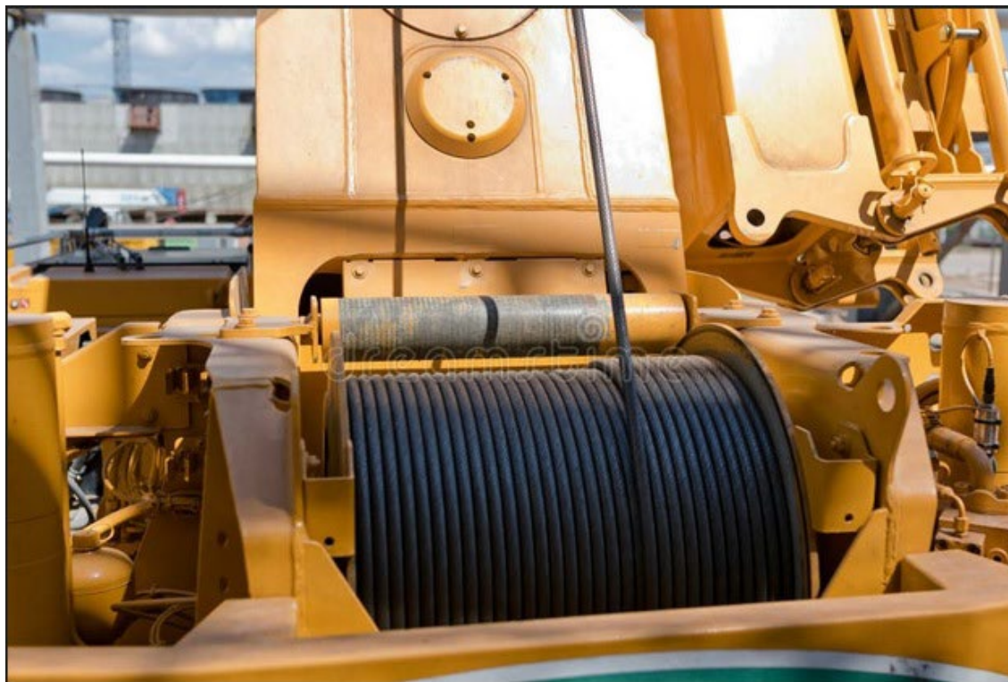
Figure 6 – depicts the winch drum inside the boom near the hydraulic brake.
