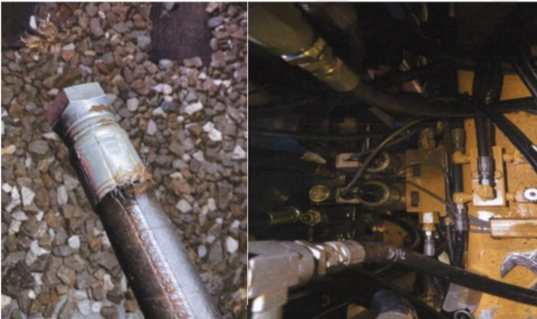
Figure 1 – Tamping Unit T004 broken hydraulic fluid line and the repaired hydraulic fluid line.
