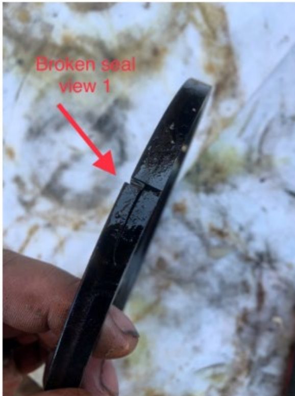
Figure 13 - Broken seal from winch brake from PM-578.
