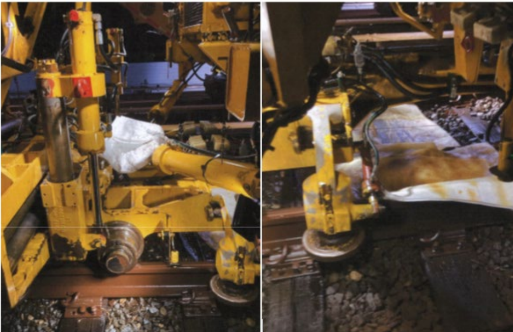
Figure 9 - Tamping Unit T004 leaking hydraulic fluid onto Absorbent pads.
