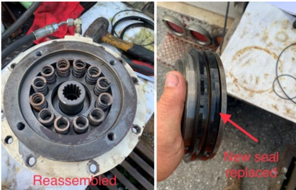
Figure 14 - Reassembled winch with new seal.
