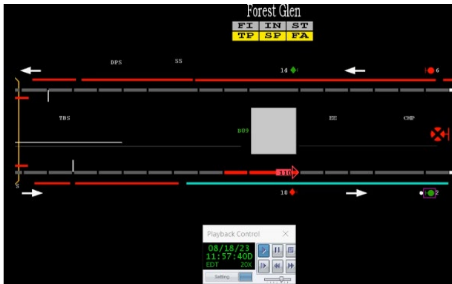
Figure 2 – Third rail power de-energized at Forest Glen Station on track 1.
