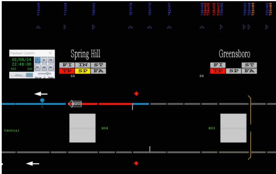
Image 11: Power was re-energized between the Spring Hill Interlocking and the end of the Greensboro Station platform limits, track 2 at 22:48 hours.
