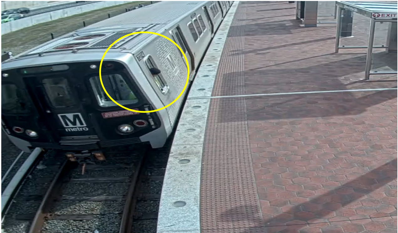
Image 1 – Train Operator looked out cab window second time prior to opening doors while the train doors were outside the platform limits.
