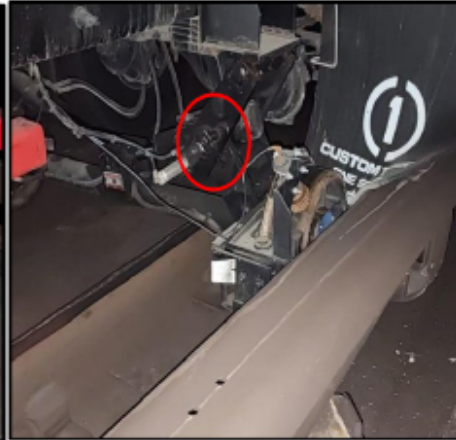
Figure 2. Right rear Locking mechanism not engaged
