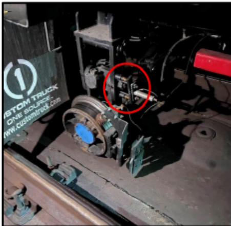
Figure 1. Left rear locking mechanism not engaged
