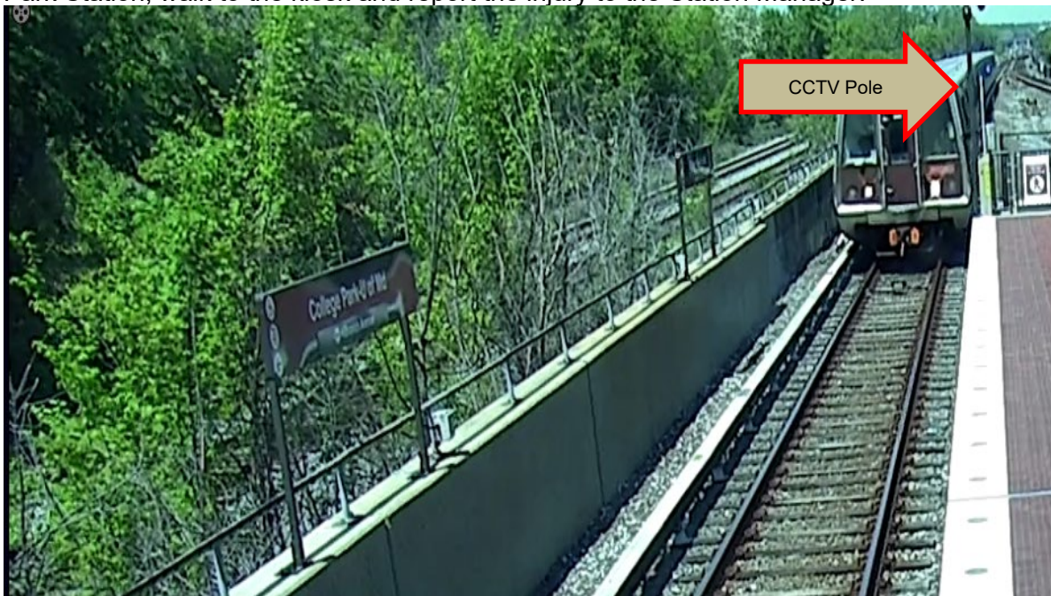
Image 2 – Employee's left arm extended out of the cab window, in close proximity to the camera pole.
