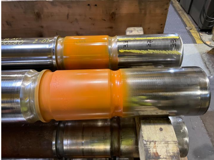
Photo #8- Re-used axles are being inspected for compliance with taper requirements. Out of compliance axles are painted orange for verification, then they are re-inspected and/or discarded.
