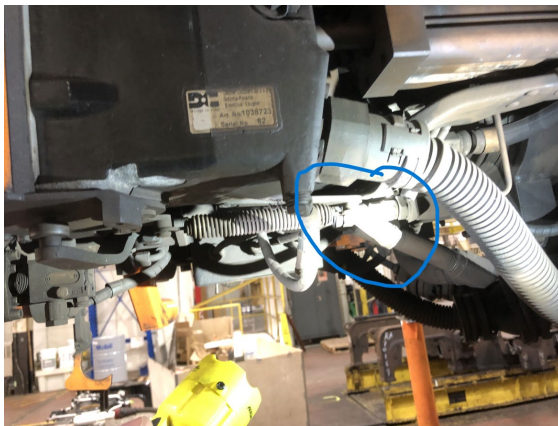
Fig 4 shows overhauled couplers with the incorrect air filters on the couplers
