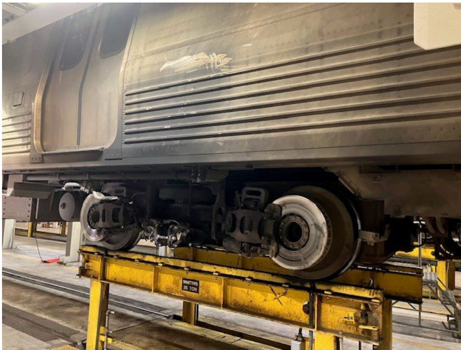
Image 15 - Shows the fire damage to the side of railcar 7663.
