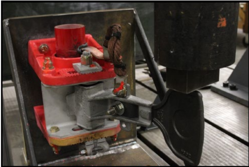
Figure 5: New collector assembly drop testing configuration
