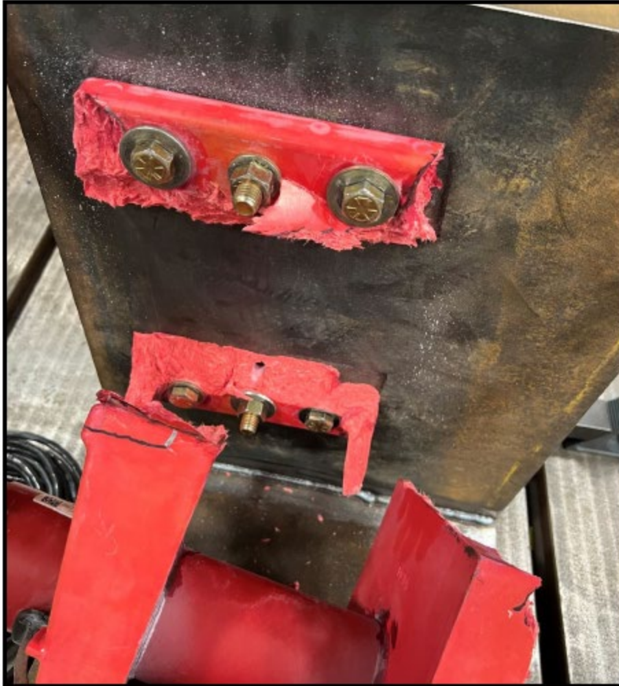
Figure 19: Additional view of the used unit failure from drop tests
