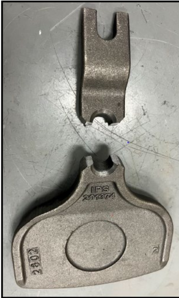
Figure 9: Typical failure mode for static loading of the shoes
