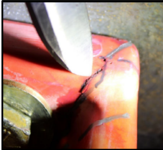
Figure 15: More crack propagation on the used assembly during the drop tests
