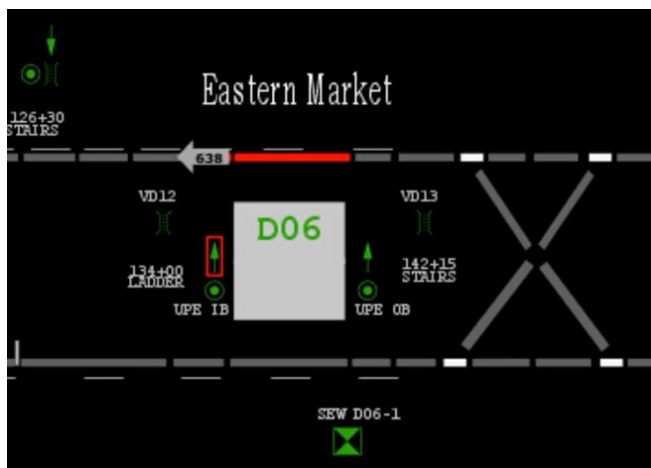
Figure 8 – Shows the Stair Fan was turned to supply.
