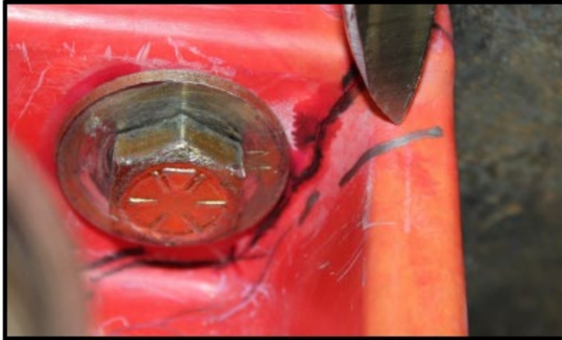
Figure 13: Crack growth on the used assembly during drop tests
