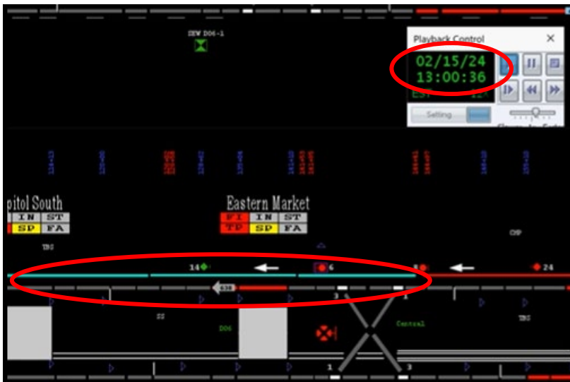
Figure 7 – Shows AIMS indicating third rail power was de-energized between Eastern Market and Capitol South Stations.
