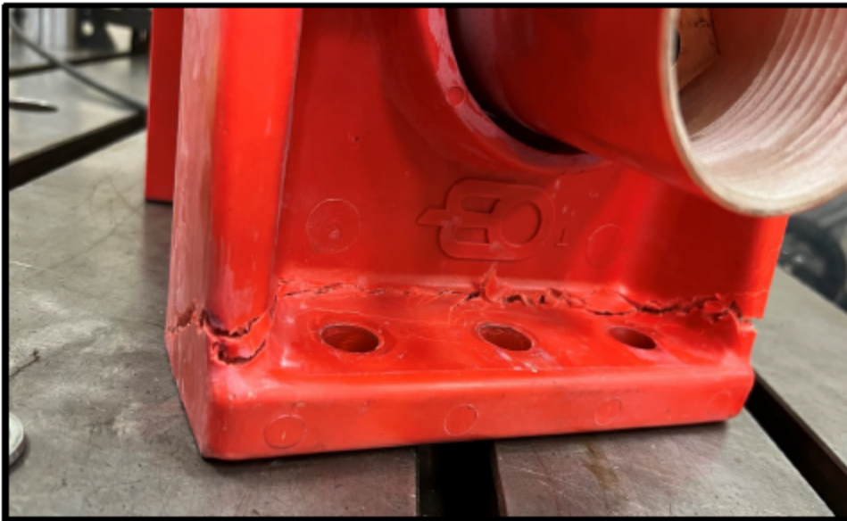
Figure 10: Failure at the base of the assembly during the assembly ultimate strength load test
