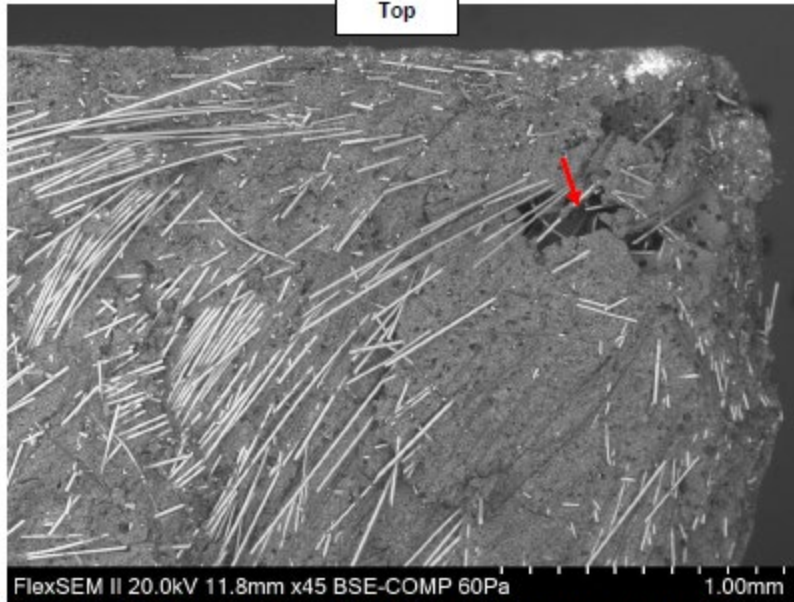
Figure 10: SEM images from the fracture surfaces of Samples 2-1 (top) 2-2 (bottom) exhibiting exposed fibers and relatively large voids along the fracture surface (red arrows).
