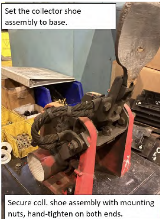
Figure 5. Mounting of collector shoe assembly.
