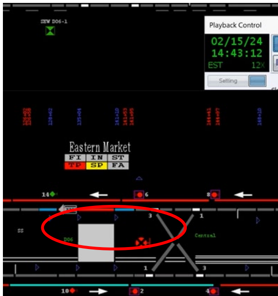
Figure 10 - Shows third rail power was restored on track 2 only to move the incident train.
