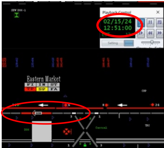
Figure 2 - Shows seconds later, third rail power was re-energized at Eastern Market Station track 2.
