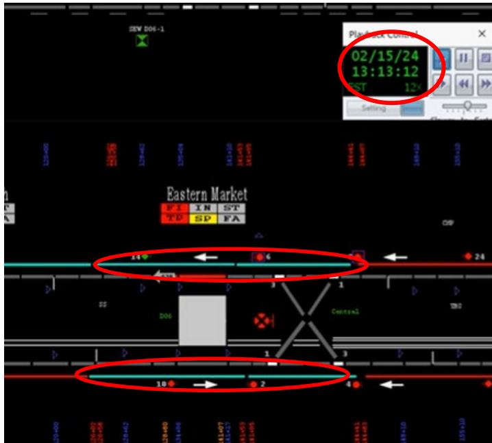
Figure 9 – Shows AIMS indicating third rail was de-energized on both tracks 1 & 2.
