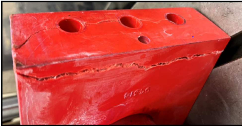
Figure 12: Failure at the base of the assembly during the ultimate strength load test
