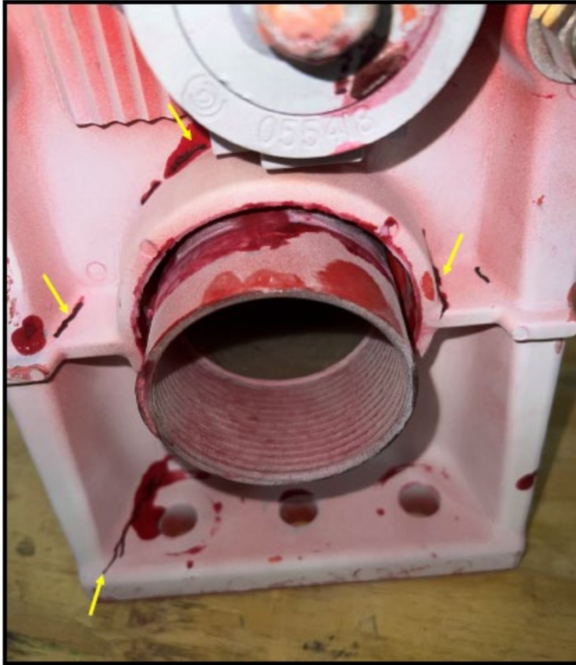
Figure 22: Second photo of dye penetrant testing used on the new assembly following the drop tests
