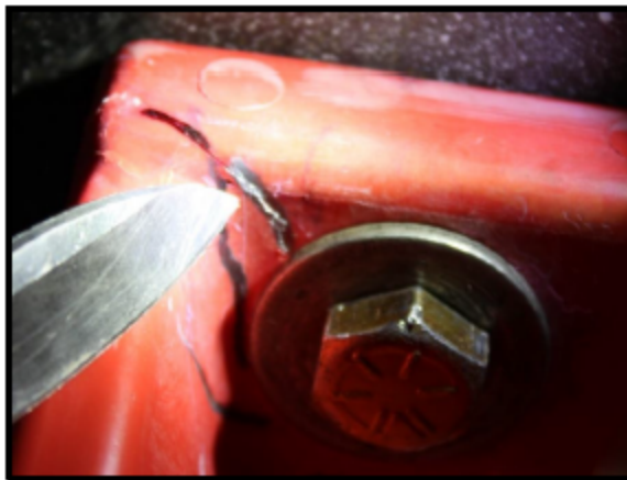
Figure 16: Additional separation observed on the used assembly during drop tests
