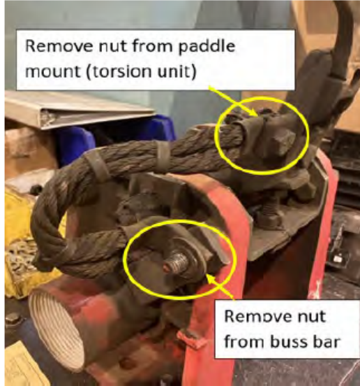
Figure 8. Removal of shunt
