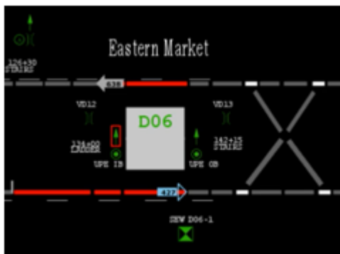
Figure 3 - UPE Inbound to the left of the station, and UPE Outbound to the right of the station set to exhaust at 12:54 hours.
