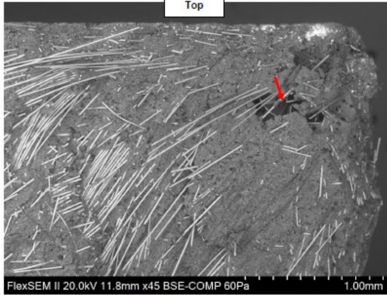
Figure 10: SEM images from the fracture surfaces of Samples 2-1 (top) 2-2 (bottom) exhibiting exposed fibers and relatively large voids along the fracture surface (red arrows).
