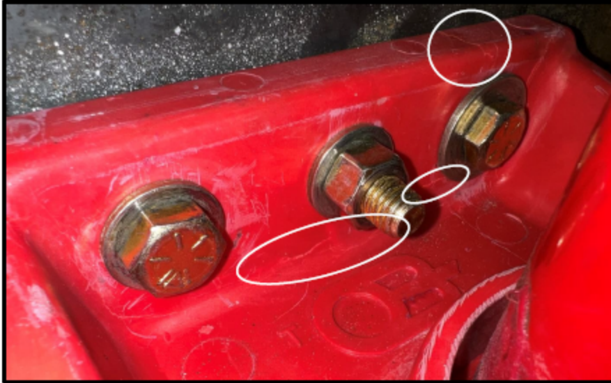
Figure 20: Crack propagation observed on the new collector assembly from drop tests
