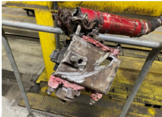
Figure 5, Circular scrapes on back of Collector Shoe Assy # 4
