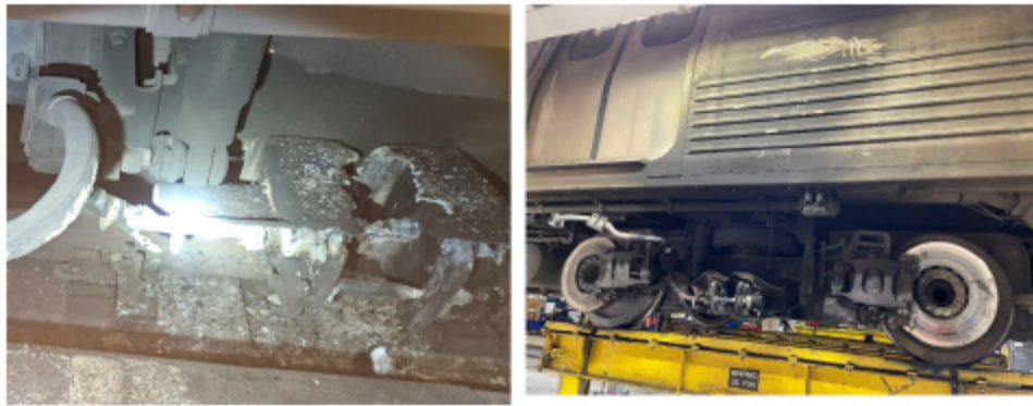
Figure 2, Car 7663 Current Collector Assembly # 1 and Fire Location
