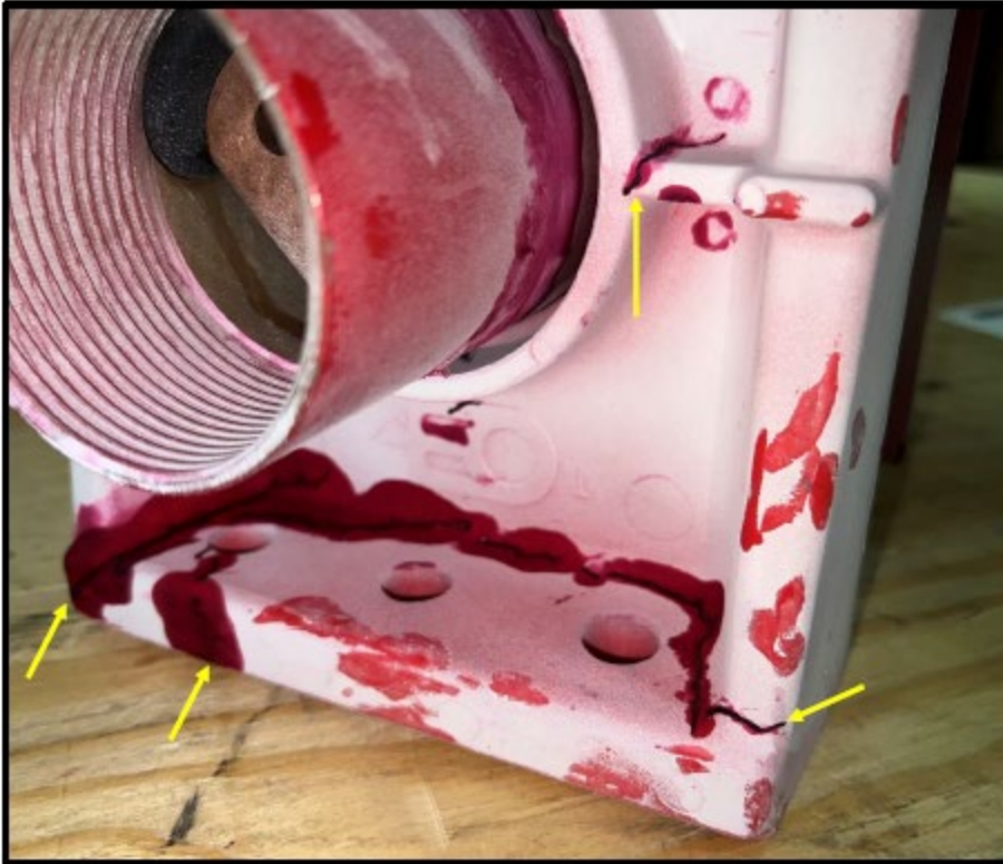
Figure 21: Dye penetrant testing on the new assembly after dynamic loading
