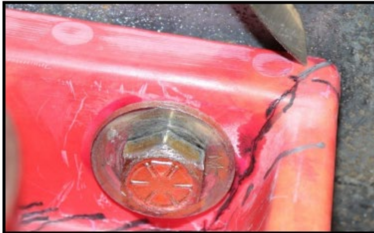
Figure 14: Separation of the surface because of crack propagation from the drop tests on the used unit
