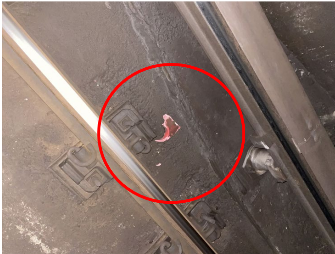
Image 16 – Image of the first fragments of the broken collector shoe assembly at CM C1 76+00 – 77+00.
