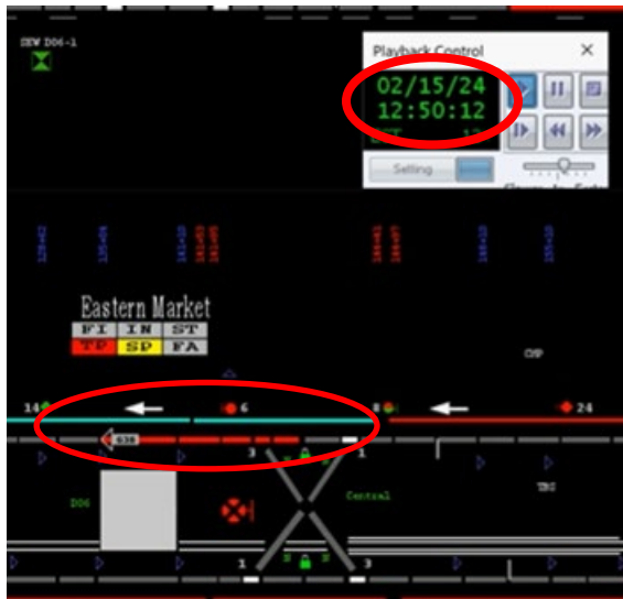
Figure 1 - Shows as Train ID 638 entered Eastern Market platform limits, third rail power dropped uncommanded.
