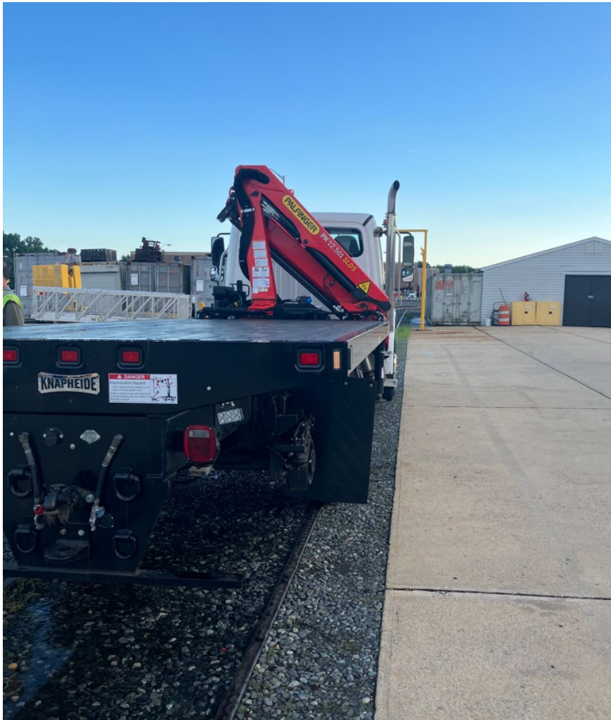
Figure 10 –Hi-Rail Unit during inspection at Greenbelt Yard can be observed with a visible lean to the left-hand side indicating uneven weight distribution.
