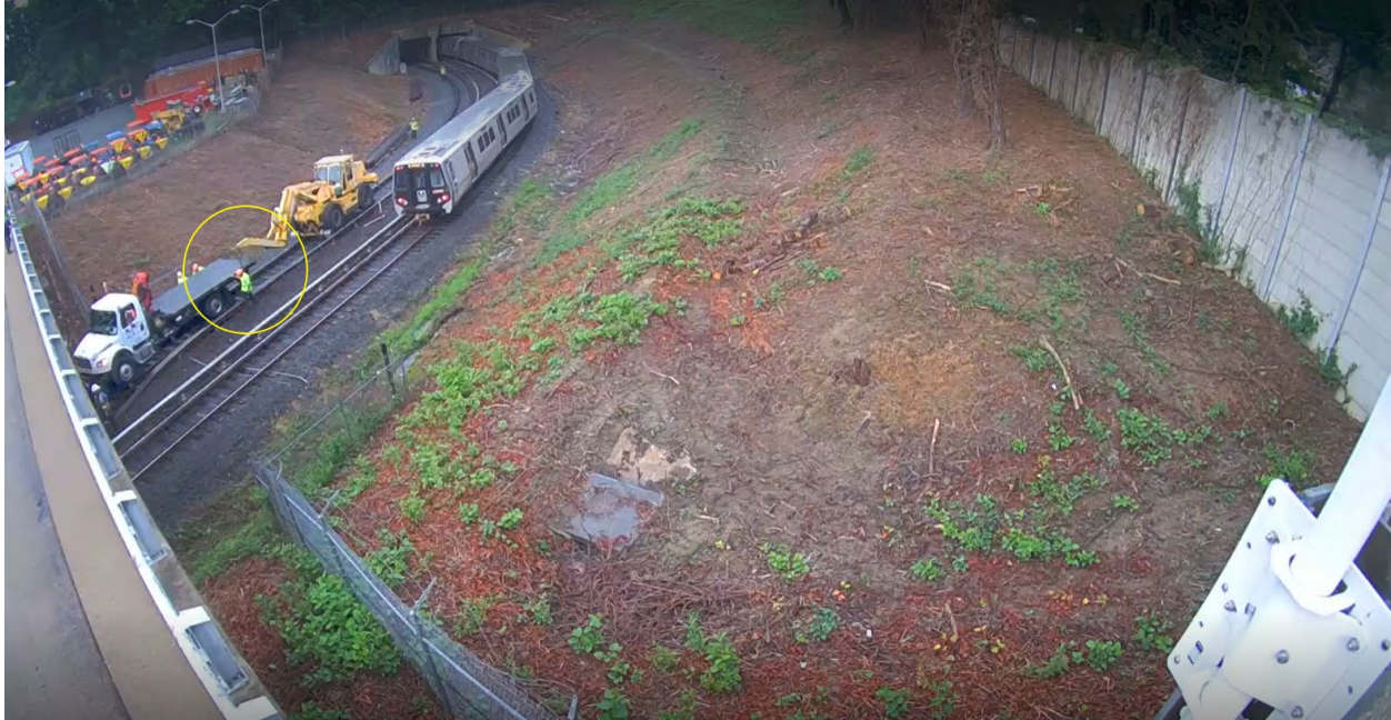
Figure 7 –The WMATA re-railing equipment can be observed lifting Unit ID CR5971's rear wheels and pushing the Unit along YL2 into West Falls Church Yard at 06:28 hours. Note YL 1 was utilized to dispatch revenue trains during the event.
