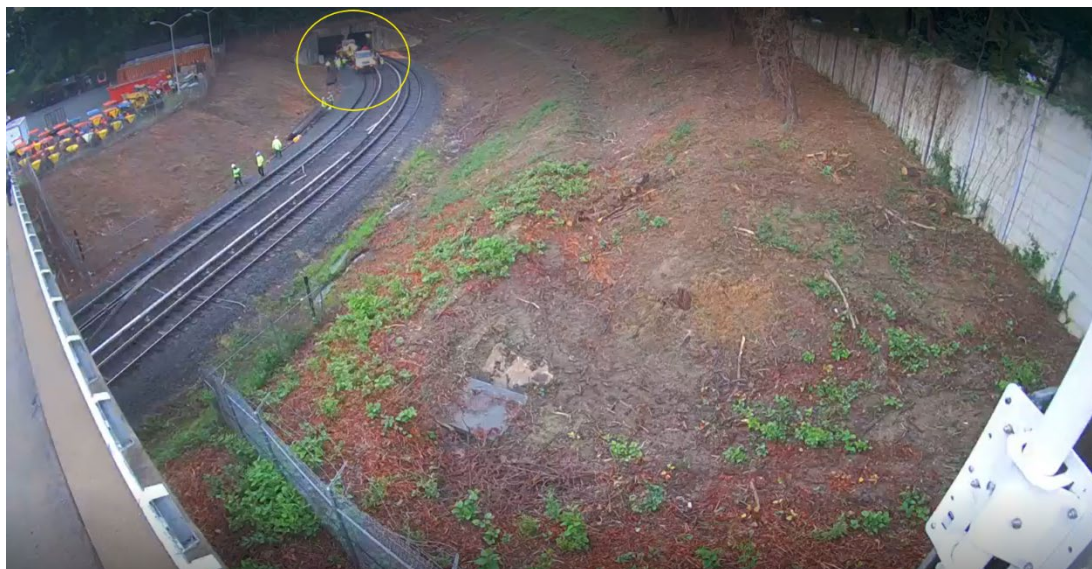
Figure 6 – The WMATA re-railing equipment can be observed lifting Unit ID CR5971's rear wheels and pushing the Unit along YL2 into West Falls Church Yard at 06:26 hours.
