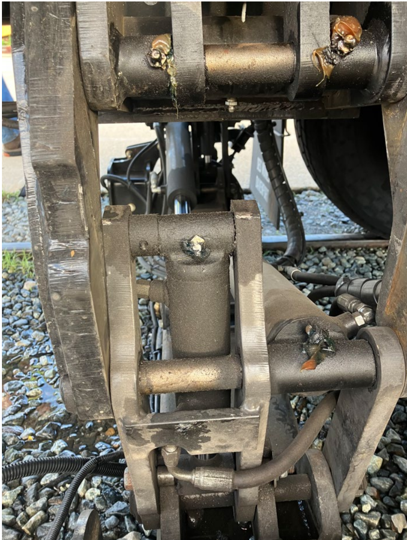
Figure 9 –Hi-Rail Unit during inspection at Greenbelt Yard had multiple defects including a shorn-off grease nipple to the rear right shock-absorber.
