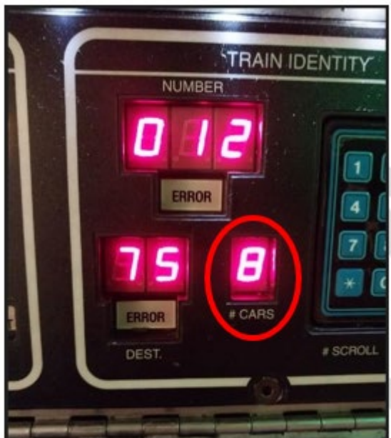
Image 7 – The Console Display Unit (CDU) shows a maximum number of 8 cars, although 10 cars were coupled together.
