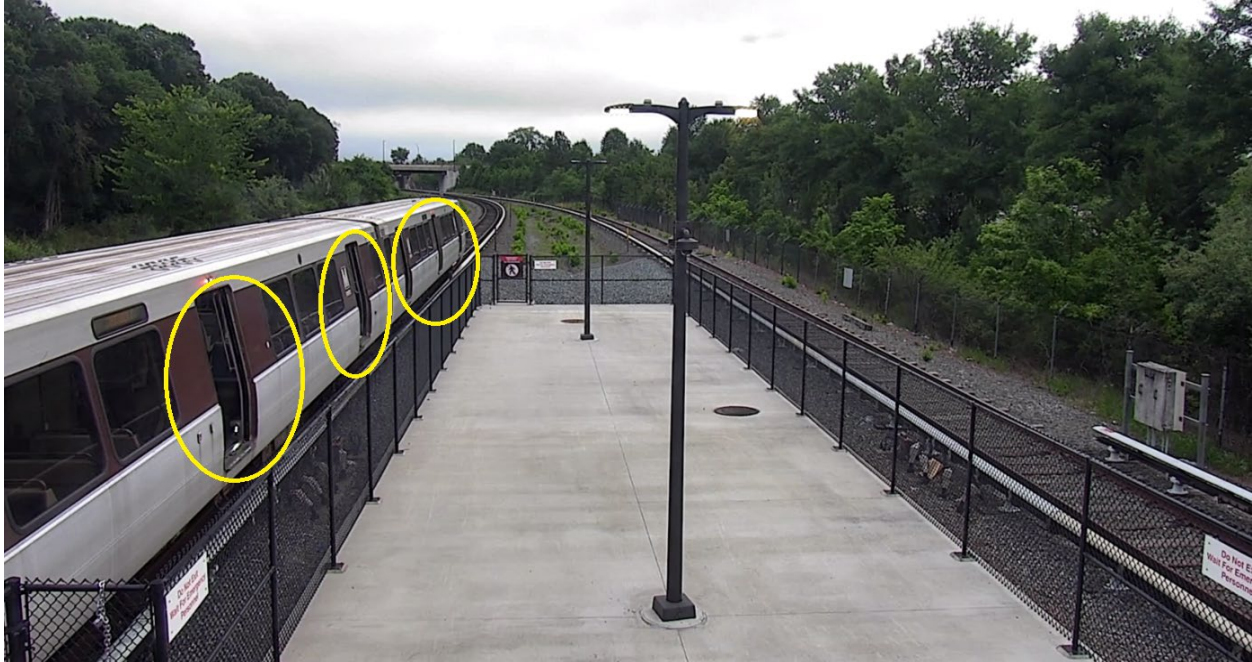
Images 3 and 4 – The platform side doors of Train ID 502 open with two cars outside the platform limits at 06:55 hours.
