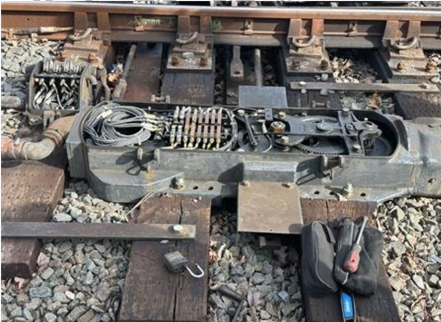
Model 6 Switch Machine lp Internal rp B98.jpg
