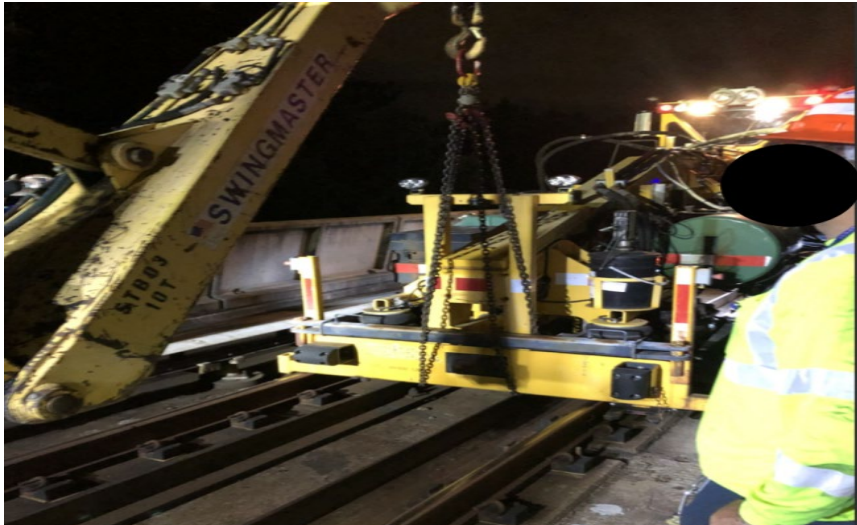
Image 5: Shows SM03 assisting with the re-railing of TR05.
