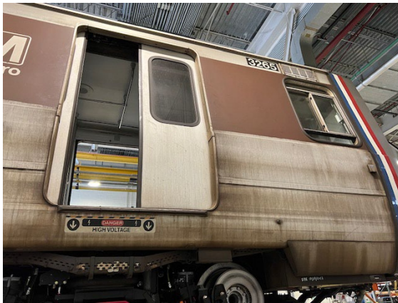
Photo 3. Railcar on lift without fall protection in place.
