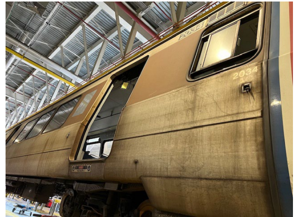
Photo 4. Railcar on lift without fall protection in place.
