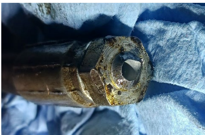
Figure 2 - Failed hose fitting.
