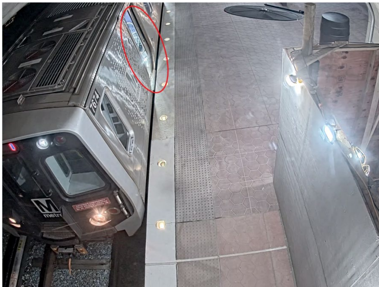
Figure 8 - depicts Train ID 140 doors opening before the RVO visually observing the platform.
