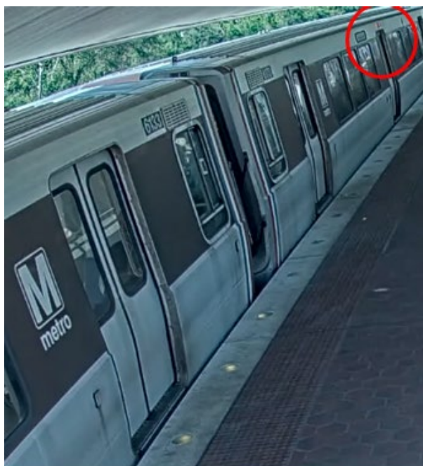
16:21:09 – the platform side doors were closed, but the door lights were still illuminated.
