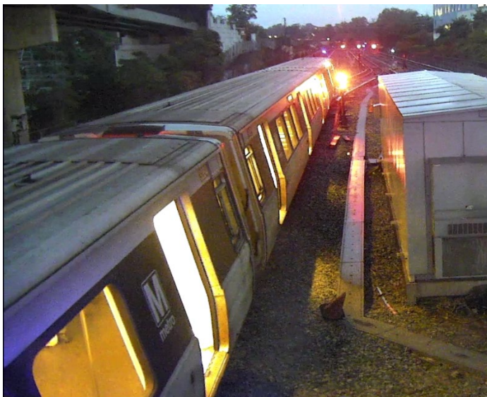
Figure 1 - (CCTV) railcars 3152 and 3153 doors open outside the platform limits.
