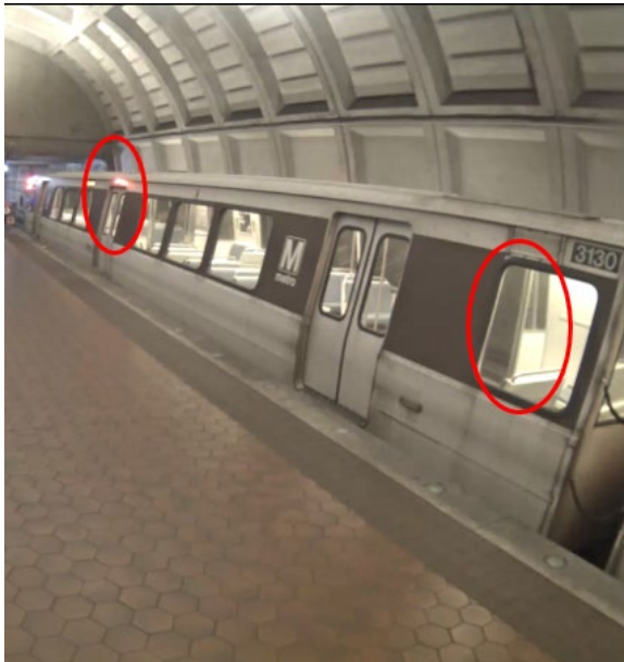
Image 2 – At 16:07:18 hours, Train ID 108 door lights were illuminated. The non-platform side doors were opened.
