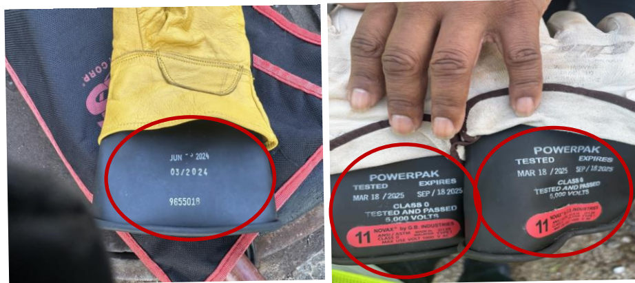
Photo 1 (left). Yellow insulated glove expired June 30, 2025.
