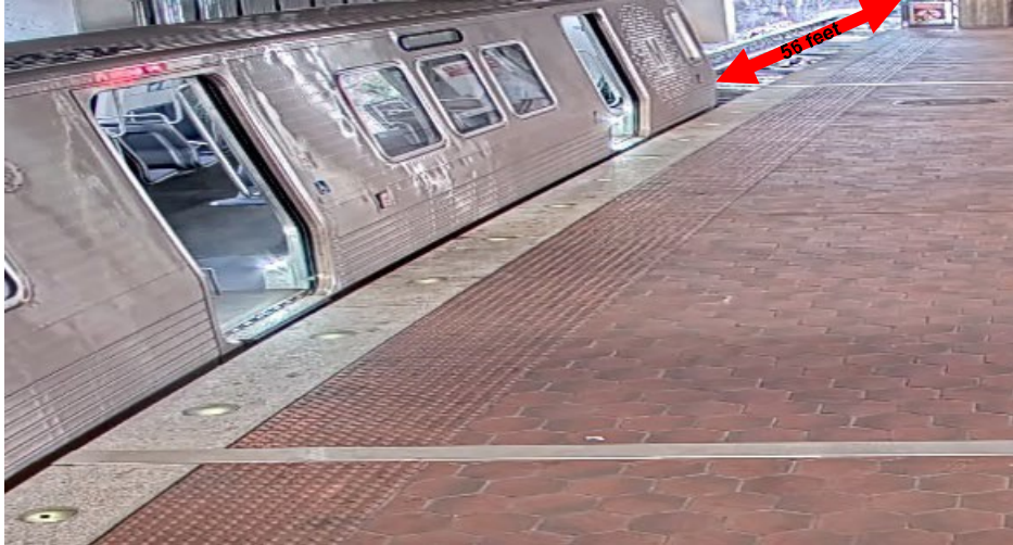
Figure 1: Train ID 404 stopped 56 feet short of the eight-car marker and serviced the station.
