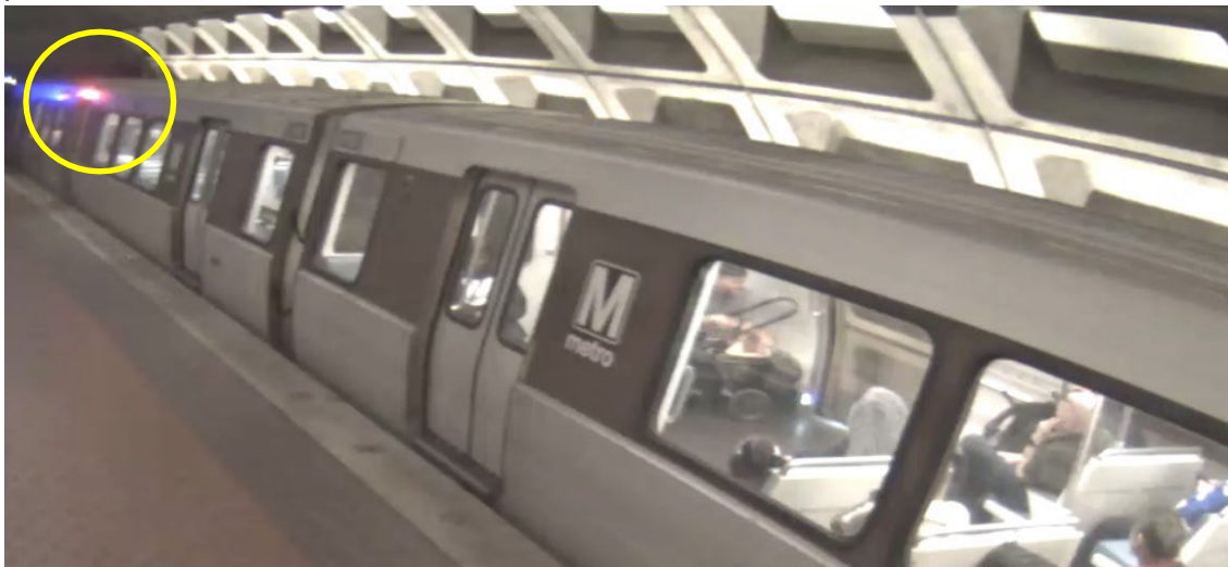
Image 3 – Depicts Door Signal Lights illuminated platform doors remained closed indicating the train doors were opened on the non-platform side.
