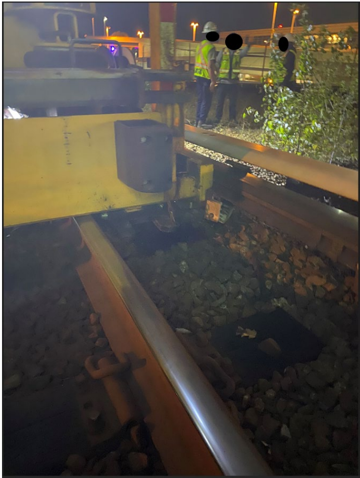
Figure 18 - Photo of TR-05 left front wheel derailed
