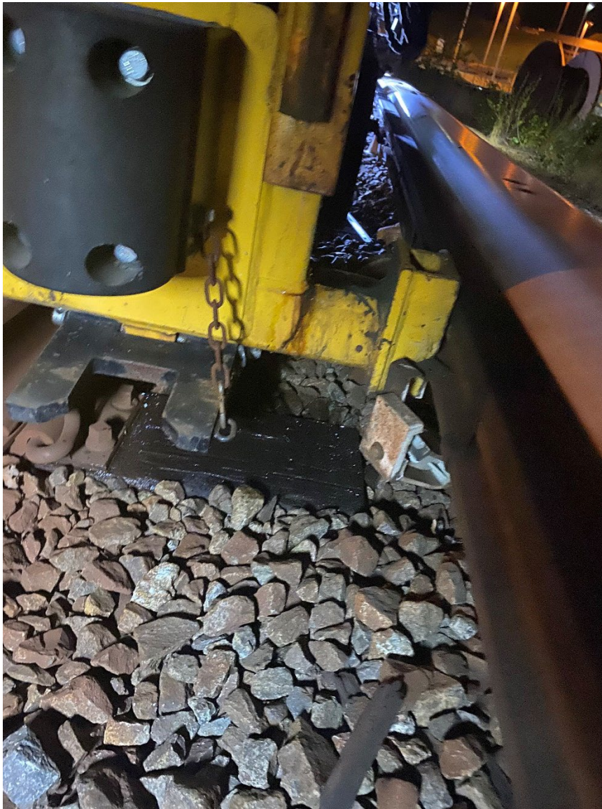
Figure 22 - TR-05 contact with the third rail and broken Insulator
