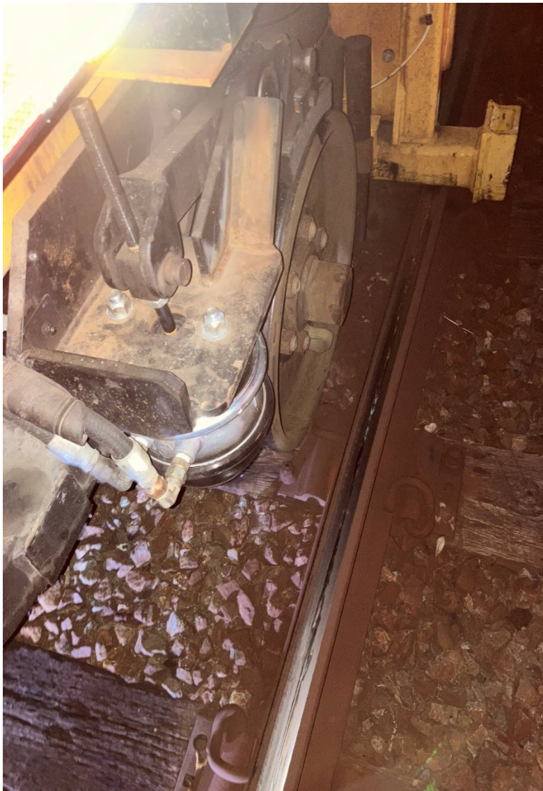
Figure 8 - Depicts the location where TR-05 is at the point of final rest with the front wheel off of the running rail.
