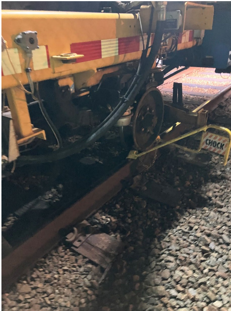
Figure 19 - depicts the rear wheel of TR-05 that remained on the running rail
