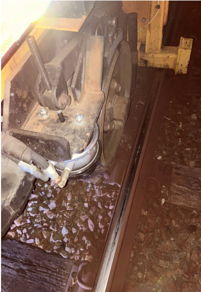
Figure 17 - Depicts the location where TR-05 derailed and scrapes on the running rail
