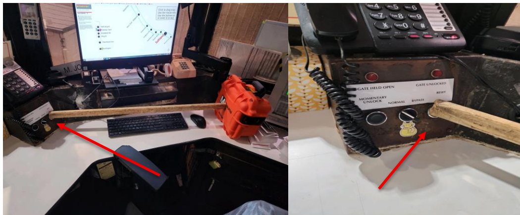
Photo 13 and 14: make-shift device to depress the "RESET" button
