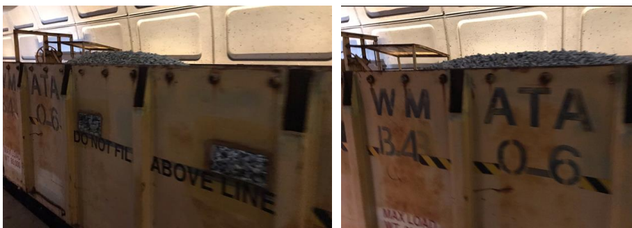
Photo 1 and 2: Overfull ballast car.
