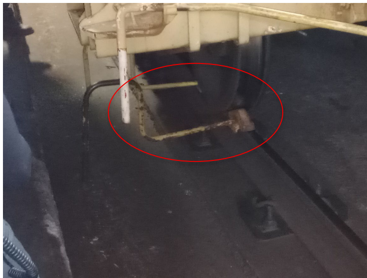
Photo 4: Wheel chock mitigation placement, rear of vehicle.
