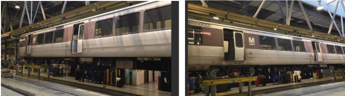
Photo 1: (left) doors open on railcar without fall protection. Photo 2: (right) Other side of vehicle doors open without fall protection.
