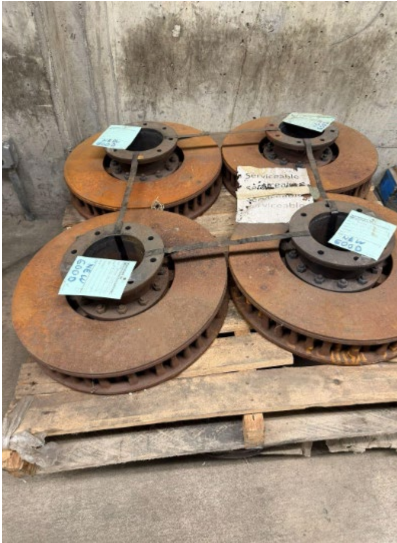
Photo 15: Brake discs marked "NEW GOOD;" however, the discs appear to be in poor condition.
