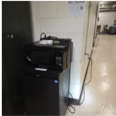
Photo 14: microwave plugged into a power strip.
