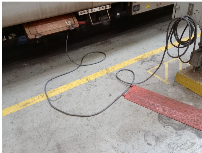
Photo 8: Shop auxiliary power cable crossing walking path without cable cover. Cover available for use.
