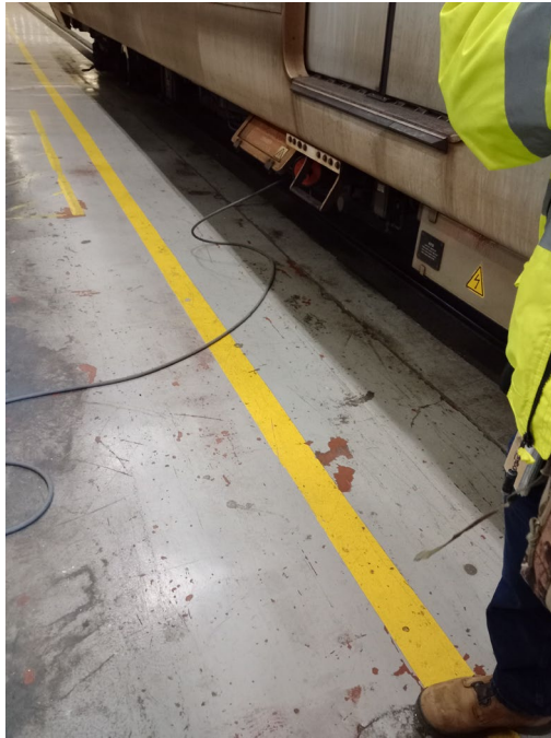
Photo 7: Shop auxiliary power cable crossing a walking path without a cover.
