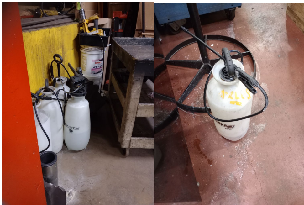
Photos 12 and 13: Handheld tank sprayers without identifying labels.
