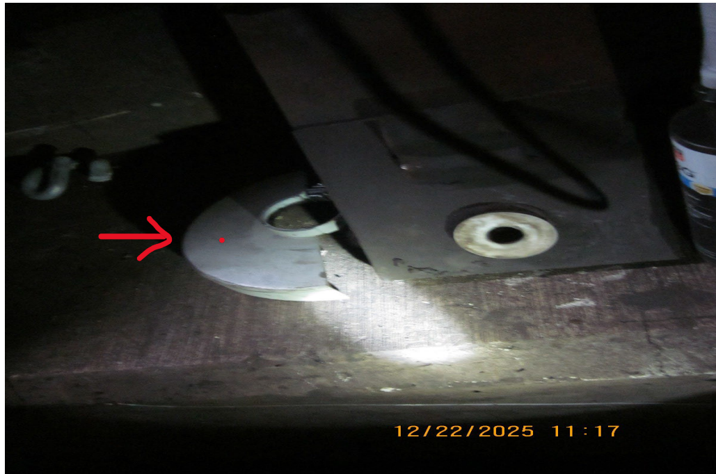
Photo 4: Shows the guard detached from the grinder.
