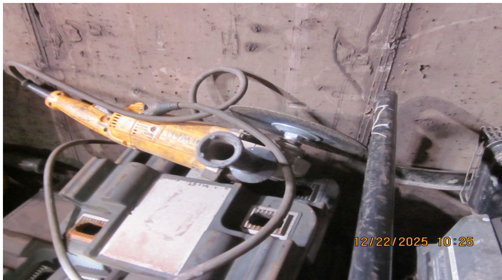
Photo 3: Grinder shown with no guard.
