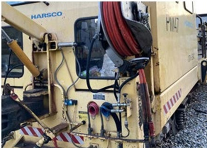
Figure 4. Damaged cut lever and hose reel noted on PM47.
