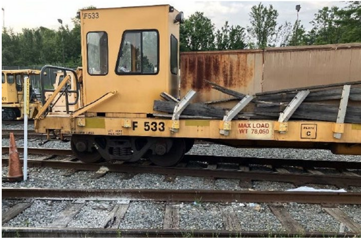
Figure 4 Damage to side pockets, side boards, and stanchions on F533
