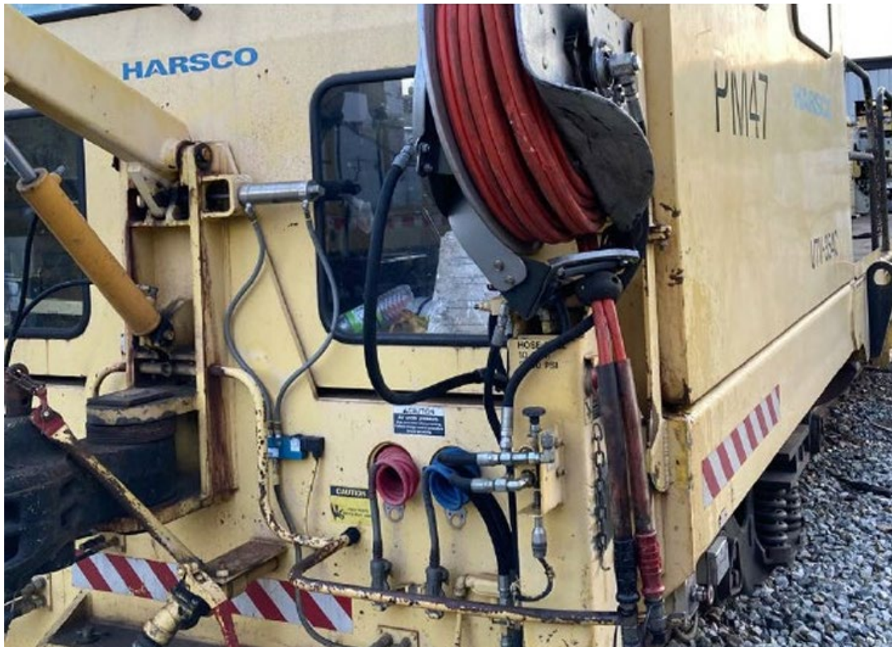
Figure 5 Damage to the cut lever and the hose reel on PM47.
