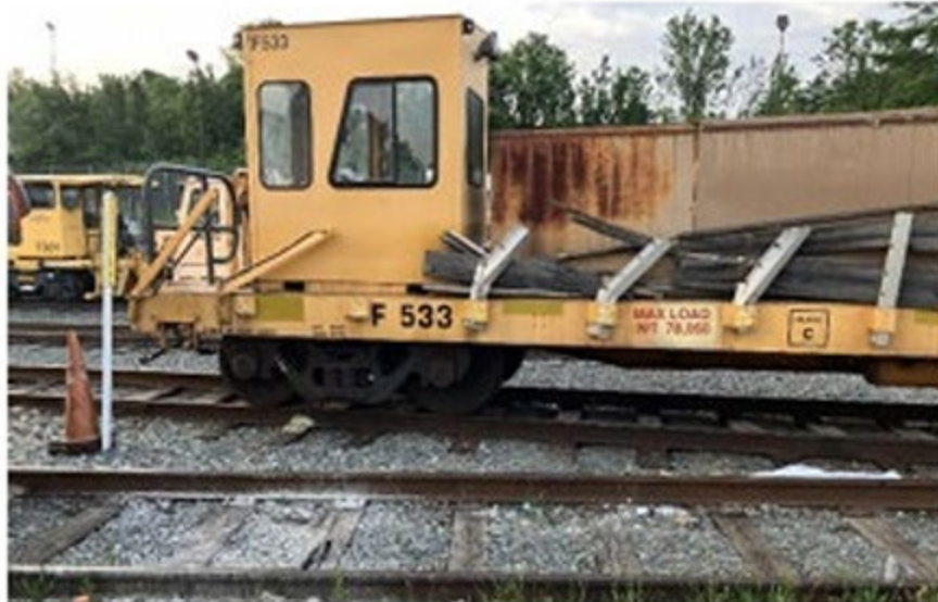
Figure 3. Damage to side pockets, side boards, and stanchions on F533.
