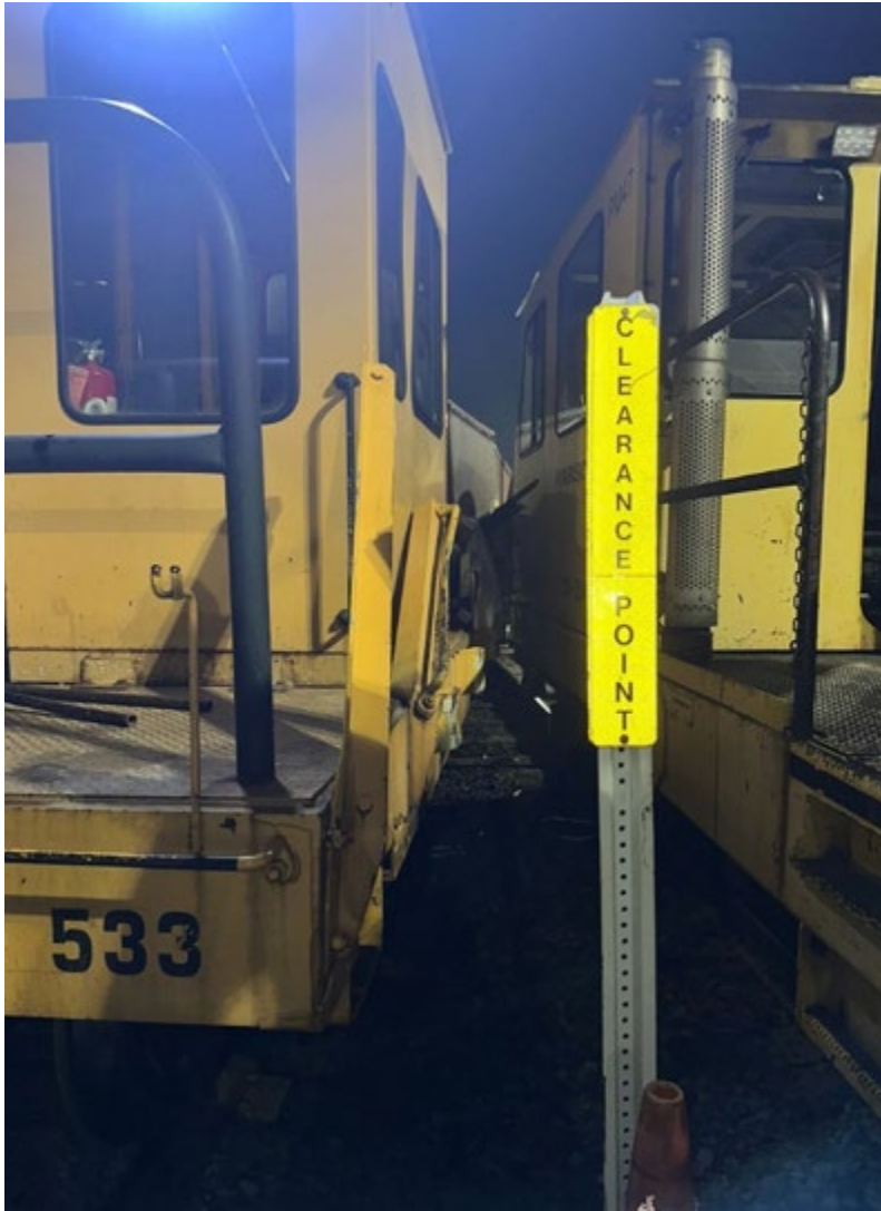
Figure 3 The clearance point sign showing PM-47 is not clear
