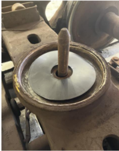
Figure 3. Circumferential damage to center pivot bowl
