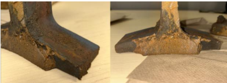
Photo 1: Failure of the weld at the base of the rail.
