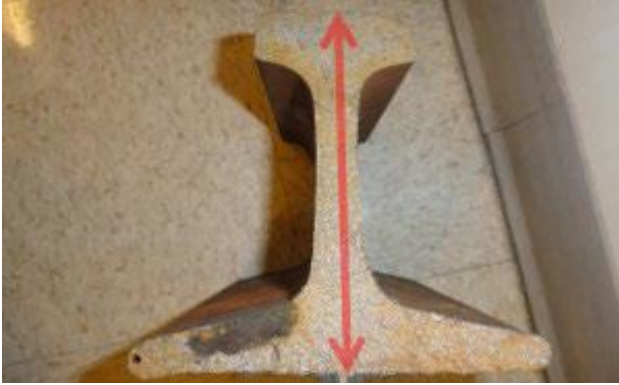
Photo 2: Shows the range that the Ultrasonic testing covers on the rail, which excludes the outside base of the rail.
