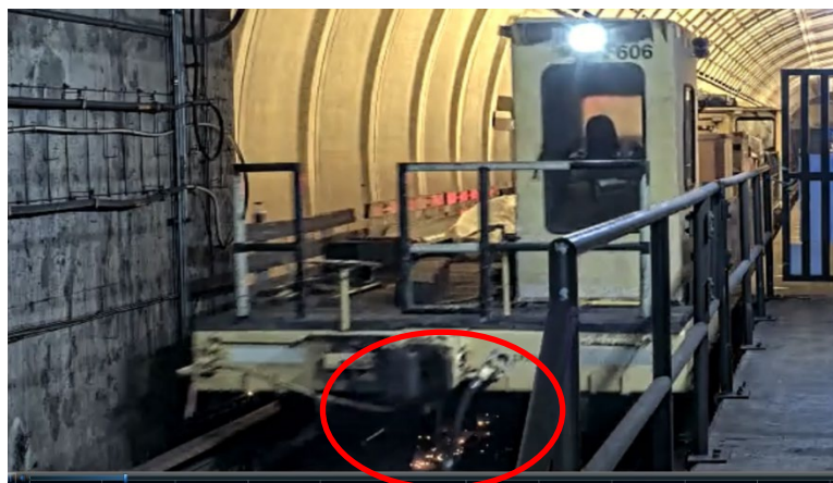
Figure 1 - This image shows sparks under the Flatcar F606 as it exits Columbia Heights Station Track 2.
