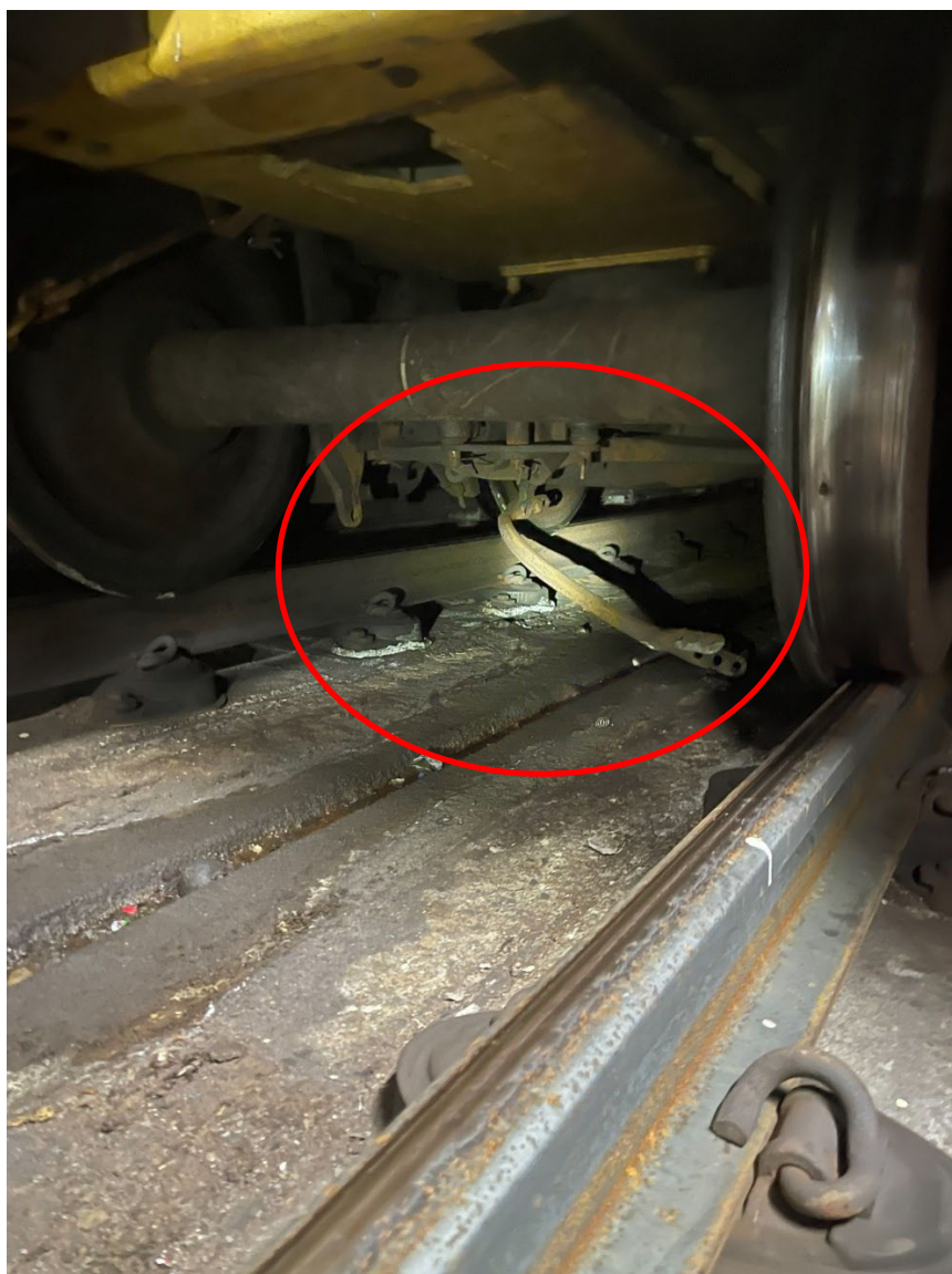
Figure 4 - Flatcar F606 hanging brake rod.
