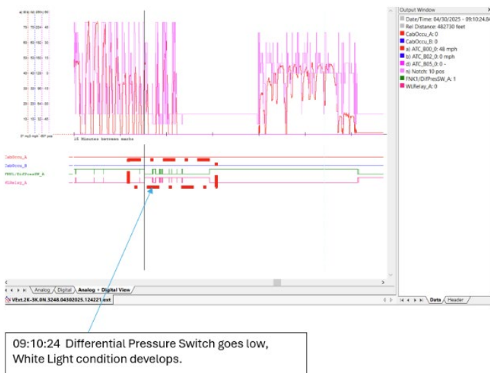
Figure 1 – Railcar 3248 VMS Analysis showing low differential pressure switch and white light condition.
