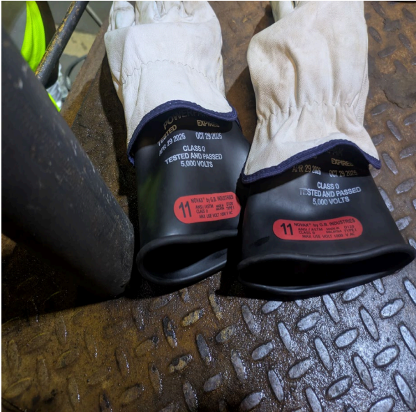
Photo 1: Third rail high voltage gloves in compliance.
