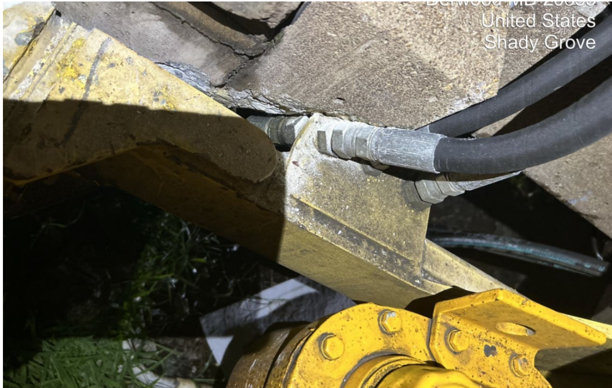
Image 2 – Image of ST-04 wedged into the concrete area beneath the platform.
