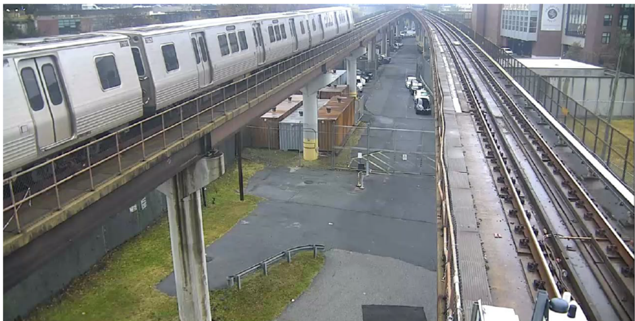
Figure 3 - Train ID 128 at a point of final rest with 3 trailing cars outside of the platform limits.
