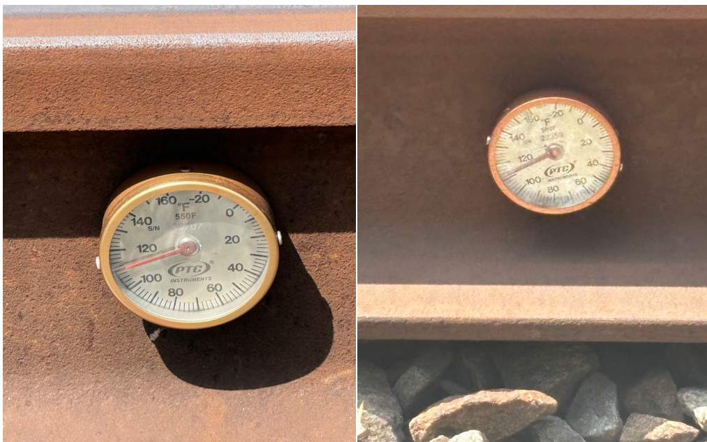
Photo 1 (left): First temperature recording at Greenbelt showing rail temperature of 110°F. Photo 2 (right): Rail temperature reading at College Park showing 112°F. (If the rail temperature reaches 135°F or higher, a system-wide above-ground speed restriction of 35mph is implemented until temperatures drop below 135°F.)
