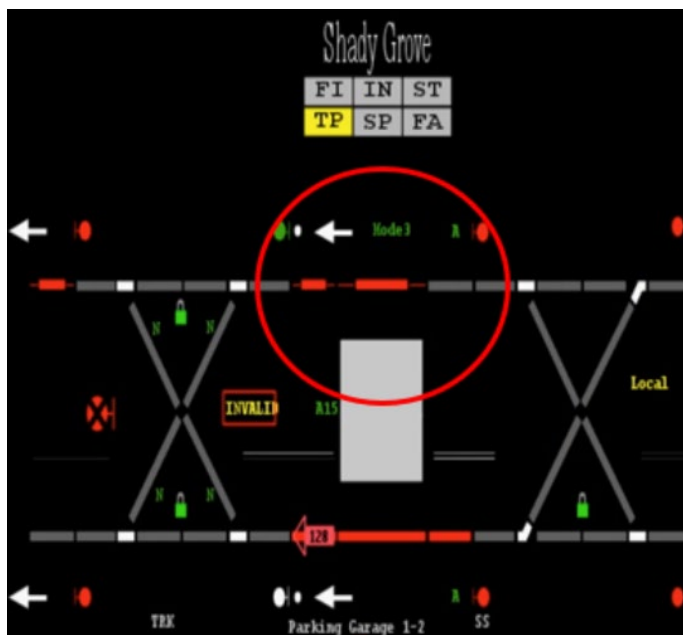
Figure 3 - (circle) depicts Train ID 124 pulled back on the platform, Track 2 at Shady Grove Station at 09:10 hours.
