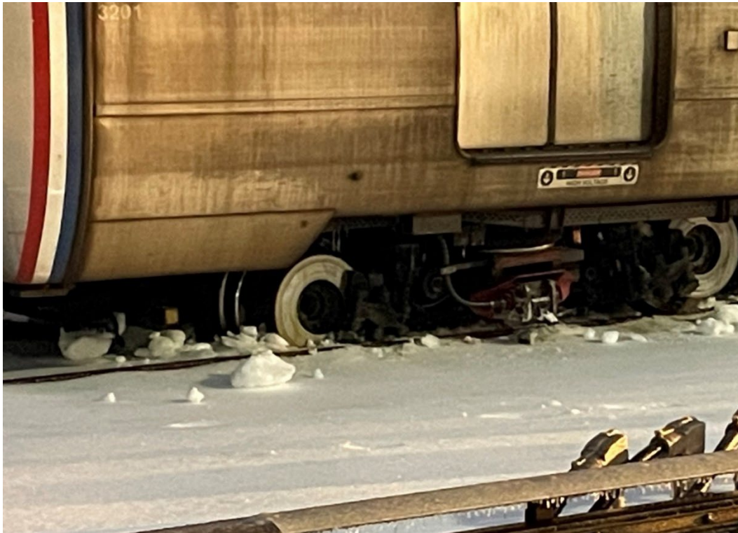
Image 3: Shows Train ID 805's wheels are off the running rails.
