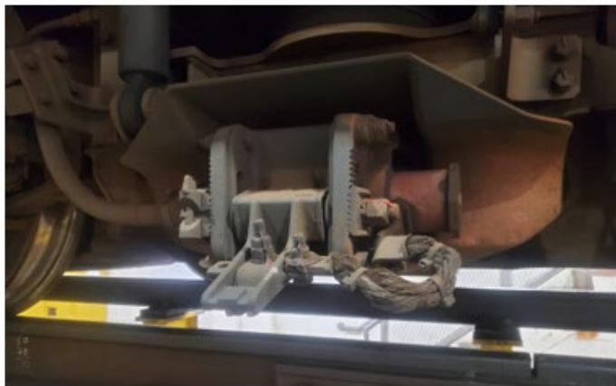
Image 5 – Photos of R7306 missing collector shoe #1; and R7307 bent left suspension reservoir draincock bracket.
