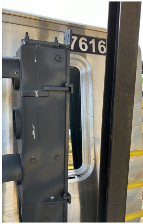
A sunshade of a randomly selected 7000 series train (L7616) was inspected for its functionality as designed. The train sunshade sporadically retracted by itself, not staying in place for appropriate use.
