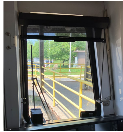
A sunshade of a randomly selected 7000 series train (L7616) was inspected for its functionality as designed. The train sunshade sporadically retracted by itself, not staying in place for appropriate use.
