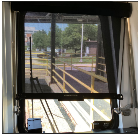
A sunshade of a randomly selected 7000 series train (L7616) was inspected for its functionality as designed. The train sunshade sporadically retracted by itself, not staying in place for appropriate use.
