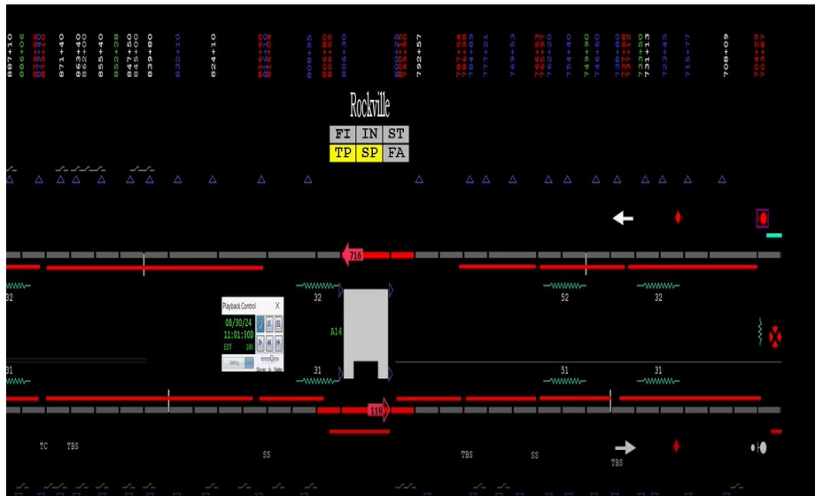
Figure 1 – Depicts third rail power re-energized at Rockville Station on track 2.
