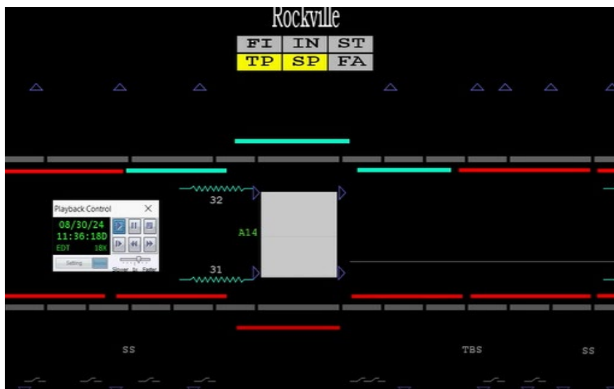
Image 5 – Third rail power de-energized at Rockville Station, track 2 to remove the customer from the roadway.
