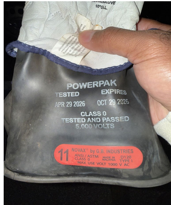
Photo 4 (left): Shows RWIC installing shunts using the required Class O insulated gloves. Photo 5 (right): Compliant Class O insulated glove.
